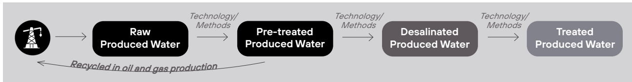
Figure 1. The produced water treatment process. Derived from Walker, Shane. "Texas Produced Water Consortium." Presentation to the Texas Desalination Association 2025 Annual Conference, slide 11, and Texas Produced Water Consortium, "Produced Water Treatment Pilot Testing: Water Quality Report," i.
