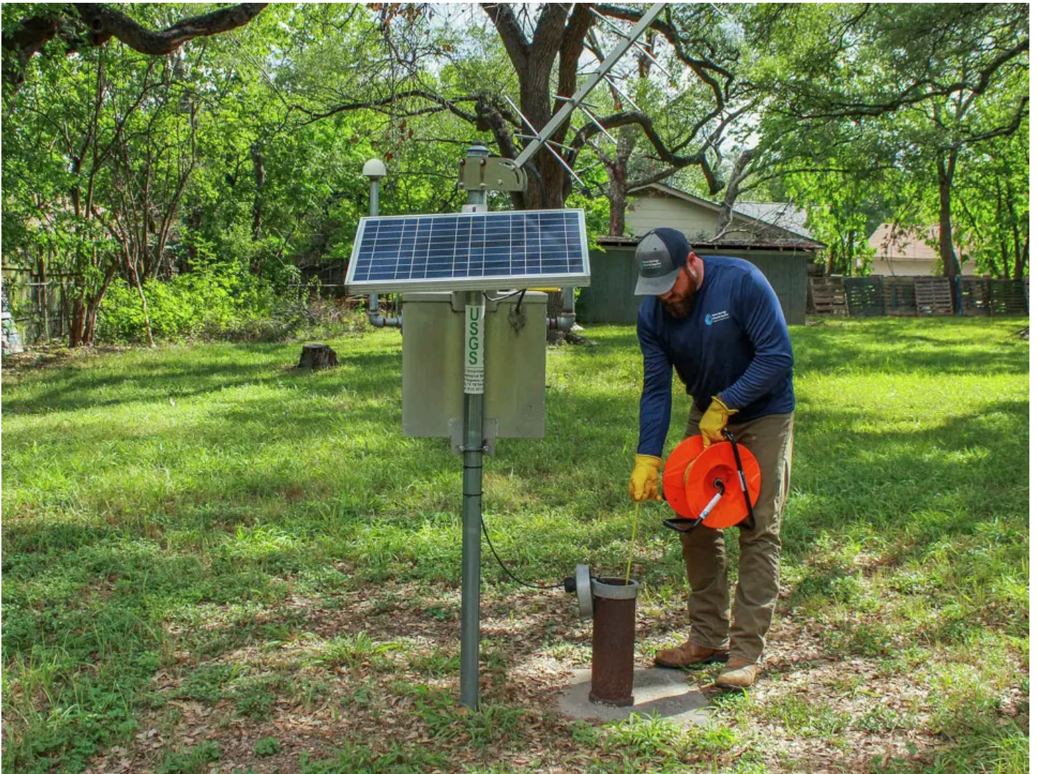
District staff measuring the Lovelady monitor well in July of 2025. Courtesy of The Barton Springs-Edwards Aquifer Conservation District
