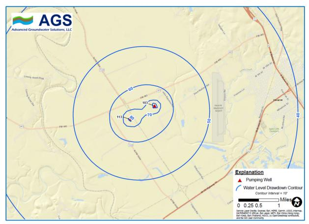
Figure 2. AGS Theis Analytical Simulated Drawdown After Proposed L. Wiese Moore LLC Pumping of 4,452 ac-ft/yr for 10-Years
