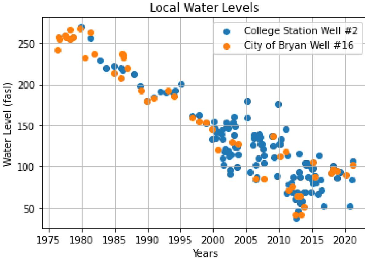
Figure 5. Water elevation hydrographs within the one-mile buffer of the proposed new wells (TWDB Groundwater Database).
