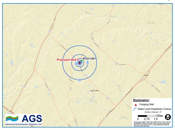
Figure 2. Analytical Simulated Drawdown Effects After Proposed Well 9 Pumping of 1,939 ac-ft/yr for 1-Year
