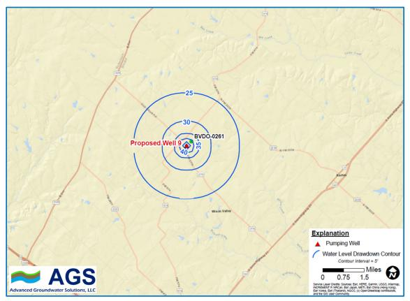
Figure 3. Analytical Simulated Drawdown Effects After Proposed Well 9 Pumping of 1,939 ac-ft/yr for 10-Years
