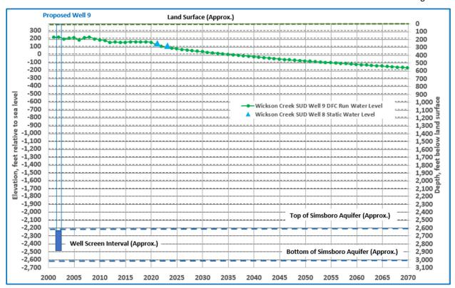
Figure 4. Projected GMA 12 2021 Planning Cycle DFC Water Level Decline at Proposed Well 9.
