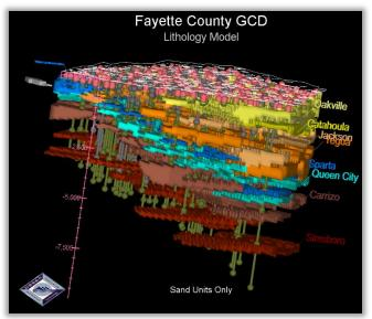
Figure 1 – Fayette County GCD 3D Hydrostratigraphic Model. Mapped sand intervals for the Oakville, Catahoula, Jackson, Yegua, Sparta, Queen City, Carrizo, and Wilcox (Simsboro) Aquifers.
