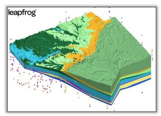
Figure 3 – Clearwater UWCD Hydrostratigraphic Model, Bell County Model Area. Color beds correspond to stratigraphic units from land surface to base of the Trinity aquifer system.
