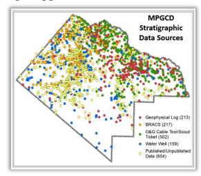
Figure 4 - MPGCD Stratigraphic Model Data Sources, organized by color and collected by ARS, LLC. Sources of data include water wells, oil and gas geophysical logs and GAM reports and models.
