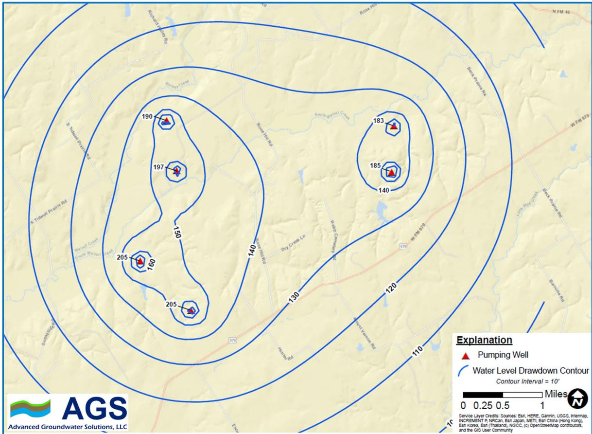
Figure 3. AGS This Analytical Simulated Drawdown After Proposed High Timber Pumping of 11,870 ac-ft/yr for 10-Years (TGI Hydraulic Properties)
