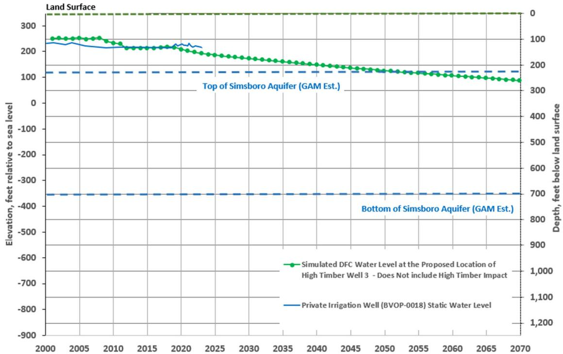
Figure 6. Projected DFC Water Level Change at Proposed High Timber Resources, L.P. Well 3
