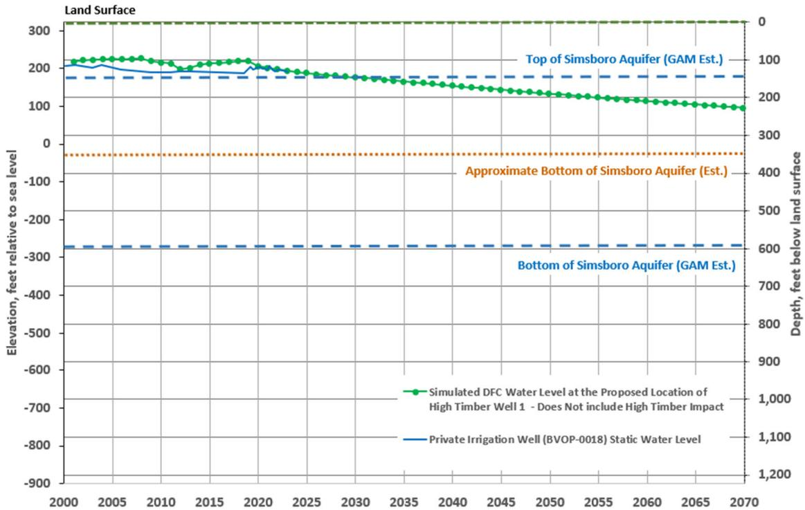
Figure 4. Projected DFC Water Level Change at Proposed High Timber Resources, L.P. Well 1
