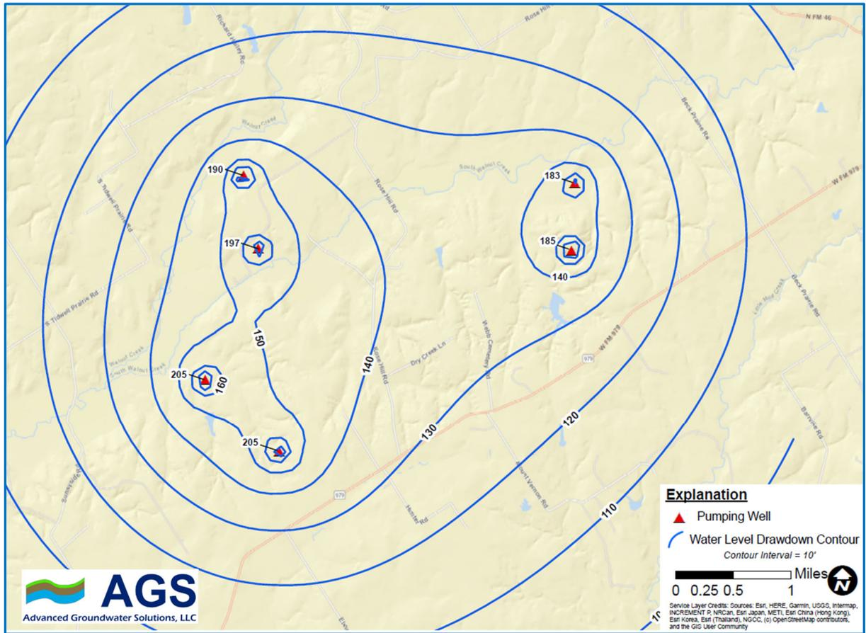
Figure 2. AGS This Analytical Simulated Drawdown After Proposed High Timber Pumping of 11,870 ac-ft/yr for 1-Year (TGI Hydraulic Properties)
