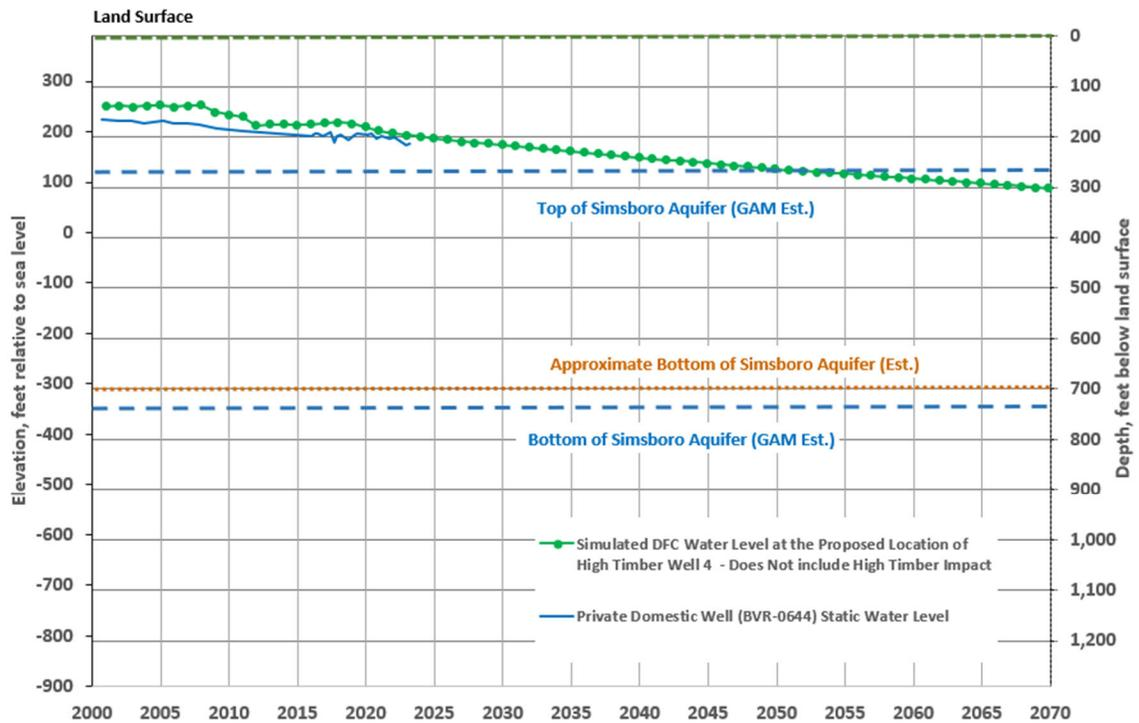
Figure 7. Projected DFC Water Level Change at Proposed High Timber Resources, L.P. Well 4
