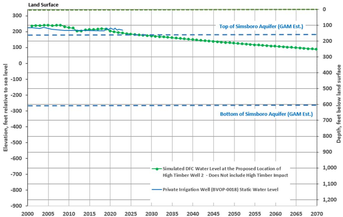
Figure 5. Projected DFC Water Level Change at Proposed High Timber Resources, L.P. Well 2
