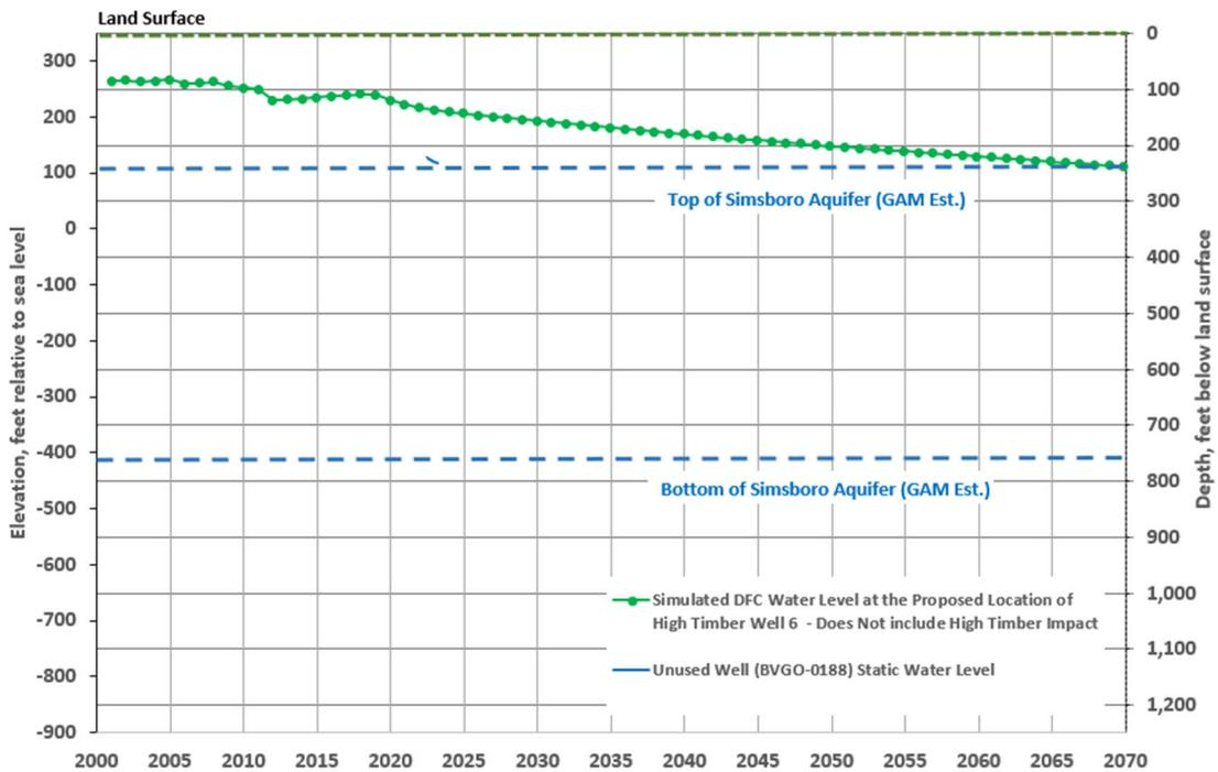
Figure 9. Projected DFC Water Level Change at Proposed High Timber Resources, L.P. Well 6
